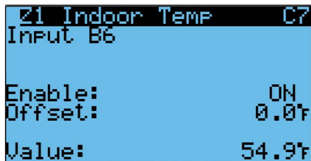
FIGURE 36 Enable/Disable Zone 1 Indoor Temperature Sensor
