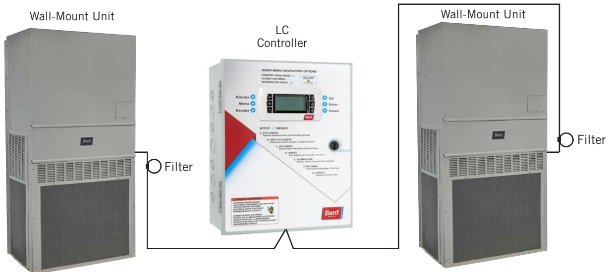
FIGURE 18 Communication Wiring (Alternate Method)
