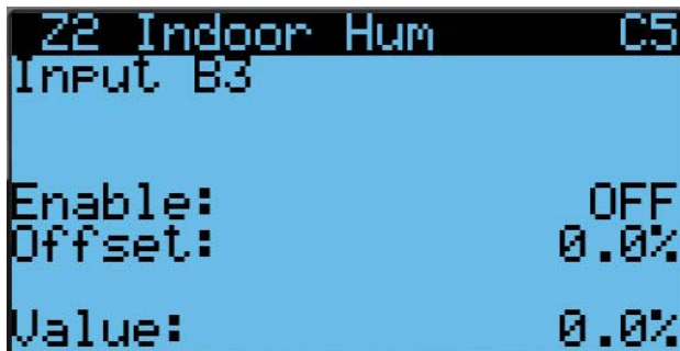
FIGURE 34 Enable/Disable Zone 2 Indoor Humidity Sensor
