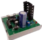
24VDC Power Supply Bard P/N 910-2198
