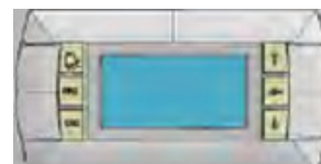
PGD Display for diagnostics and commissioning Bard P/N 8301-053
