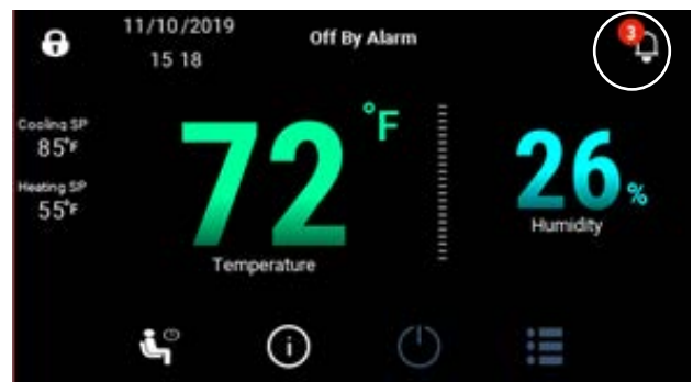
FIGURE 19 Active Alarms Displayed on Main Screen
